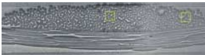
Figure 1. Cross-section of glass reinforcement in epoxy
