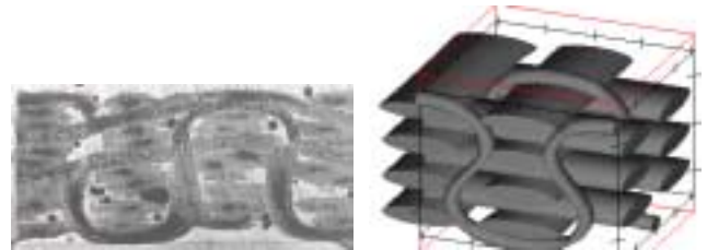
Figure 10. Typical deformed Z-yarns (cross-section and computed) in 3D fabrics
